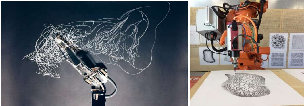
Robots Drawing – left:light source on end of arm recorded with extended exposure. Right: Scribing a pattern
